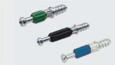
Coloured plastic sleeves in easy-to-grip fluted design indicate dowel lengths. Green (dowel length 20 mm) for Rastex 15, blue (dowel length 24.5 mm) for Rastex 25 and black (dowel length 30 mm) for Rastex 15.
