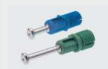
Fast, toolless installation, simply presses by hand into the hole in the carcass side. Easy to tell apart with coloured expanding elements for 8 mm (blue) and 10 mm (green) drill holes.
